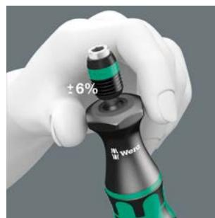
These torque screwdrivers are supplied with a fixed pre-set torque value. This is ideal for all applications that require constant, identical torque. They feature a pre-set torque range of 0.3 Nm to 4.0 Nm (adjustable between 0.3 Nm – 8.8 Nm), two different handles, measurement accuracy of ± 6 % and Rapidaptor chuck technology for rapid bit change.
