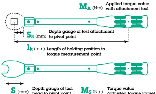
When ordering, please state the desired pre-set torque and the depth gauge size "S" of the attachment tool used.
