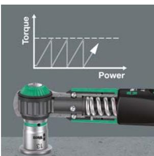
The Safe-Torque torque wrench is equipped with a slide-over mechanism. Once the set torque value has been reached, the tool cannot be overtightened, so that excessive torque cannot be applied.
